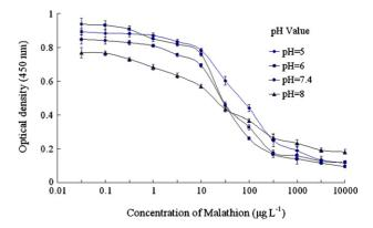
Fig. 3 – ELISA competitive curves of malathion prepared in PBS buffer containing various pH values. Data represent mean  $\pm$  S.D. of three experiments on the different days. Reagent concentrations: coating antigen II-OVA<sup>a</sup> (2  $\mu$ g mL<sup>-1</sup>); antiserum 3055 (1:6400); goat anti-rabbit IgG–HRP (1:5000).
