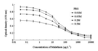
Fig. 4 – ELISA competitive curves of malathion prepared in PBS buffer containing various concentrations of ionic strength. Data represent mean  $\pm$  S.D. of three replications on the different day. Reagent concentrations: coating antigen II-OVA<sup>a</sup> (2 µg mL<sup>-1</sup>); antiserum 3055 (1:6400); goat anti-rabbit IgG–HRP (1:5000).
