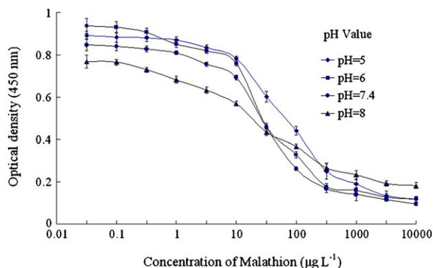
**Fig. 3 – ELISA competitive curves of malathion prepared in PBS buffer containing various pH values. Data represent mean ± S.D. of three experiments on the different days. Reagent concentrations: coating antigen II-OVA<sup>a</sup> (2 μg mL<sup>-1</sup>); antiserum 3055 (1:6400); goat anti-rabbit IgG–HRP (1:5000).**
