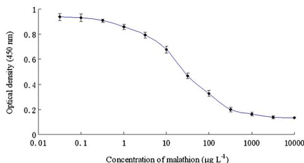
**Fig. 5 – ELISA inhibition curve of malathion. Data represent mean  $\pm$  S.D. of three experiments on the different days. Reagent concentrations: coating antigen II-OVA<sup>a</sup> ( $2 \mu\text{g mL}^{-1}$ ); antiserum 3055 (1:6400); goat anti-rabbit IgG–HRP (1:5000).**
