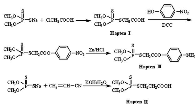
**Fig. 1 – Synthetic route for Hapten I, II and III.**
