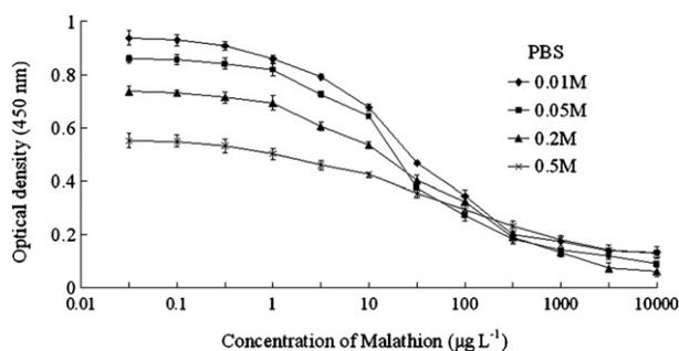
**Fig. 4 – ELISA competitive curves of malathion prepared in PBS buffer containing various concentrations of ionic strength. Data represent mean  $\pm$  S.D. of three replications on the different day. Reagent concentrations: coating antigen II-OVA<sup>a</sup> ( $2 \mu\text{g mL}^{-1}$ ); antiserum 3055 (1:6400); goat anti-rabbit IgG–HRP (1:5000).**
